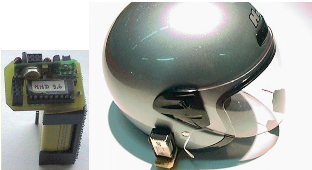
Figure 5 The HHD device and the biosensor helmet. The HHD device is mounted on the side of the helmet while four sensors are mounted inside.
