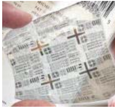
Figure 3. Printed transistor for RFID on transparent sheet
