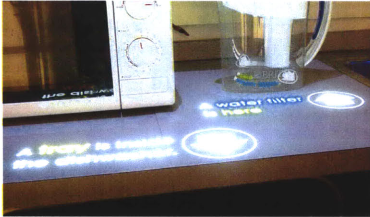
Figure 4-4. Smart indicators are projected on the countertop to let subjects understand what they can do at certain locations.
