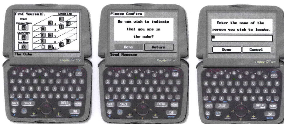
Figure 4-10: PageWriter 2000 custom applications for Junior Summit. The leftmost image shows the interface used for delegates to indicate which room they were located within the Media Laboratory or the hotel. The center image shows a confirmation screen verifies that the delegate indicated the correct room. The rightmost image shows the interface the delegates used to locate other delegates.
