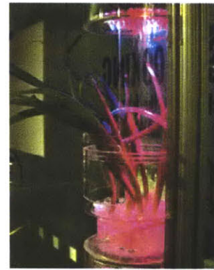
Mr. Basil, the first prototype of Living Food, is a blender-sized acrylic tube with LED array (top) and plant gel reservoir (bottom).
