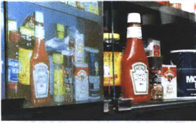
A two-dimensional projection of the cabinet's contents can reveal more than glass doors: at an oblique angle the bottle of Mrs. Dash next to the ketchup is invisible through the glass door (right), while in the projected view it is clearly visible (left).
