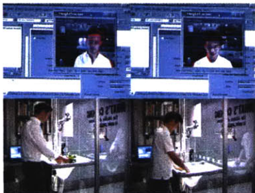
Up+Down Sink height tracking program (above) and two different heights (below).
