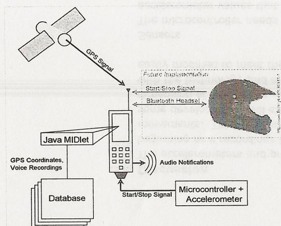
**figure 2.** System diagram for both the current and future implementation of the location-based notification system.
