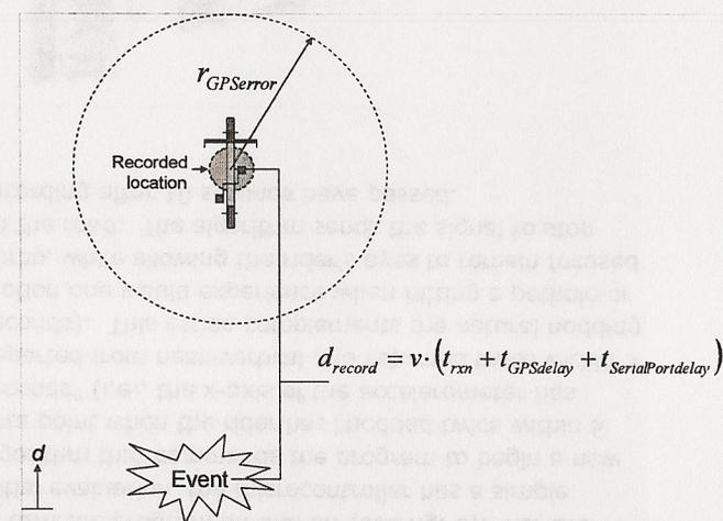
**figure 4.** Decomposition of the distance at which data is recorded, with respect to an event or location of interest.
