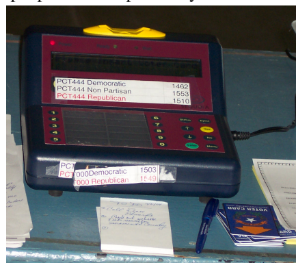
Figure 8. Card Activator labeling modified by poll worker to put provisional numbers out of the way.
