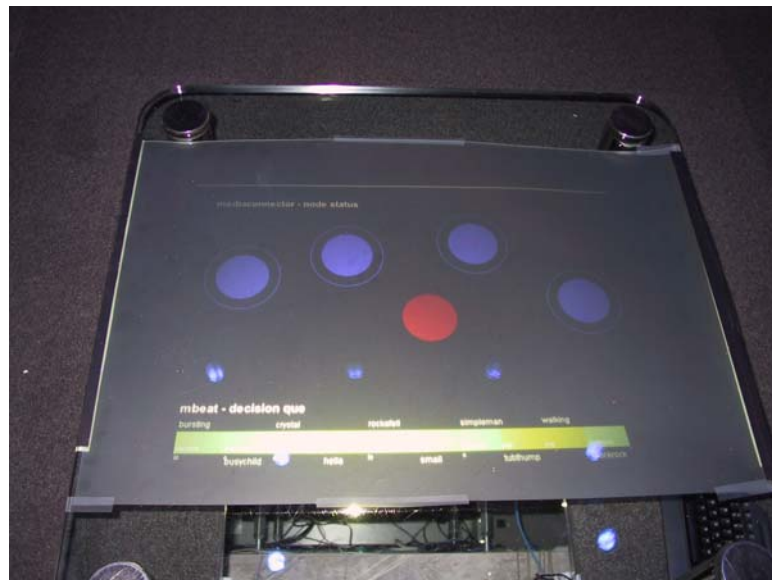
Figure 5.4 The MBeat visualization table, implemented to gain perspective into what decisions it is making. It aided debugging and also provided useful feedback to viewers.
