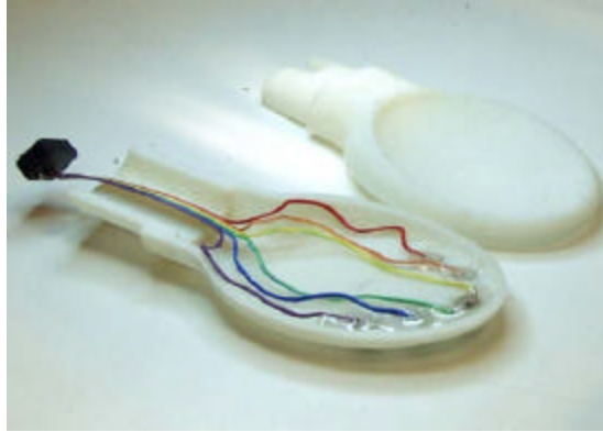
Figure 6: A 3D-printed model of the final design. Holes were intentionally left to allow rooms for sensors to be attached.
