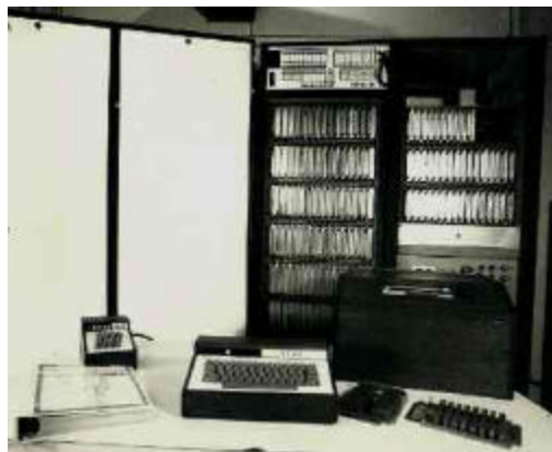
Figure 8: Electronic Computing Home Operator, ECHO, is designed and built by Jim Sutherland in 1966.
