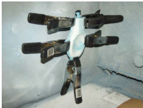
Figure 11: Filled mold in fume hood. The cramps hold the two pieces of the mold together while the silicone is curing.
