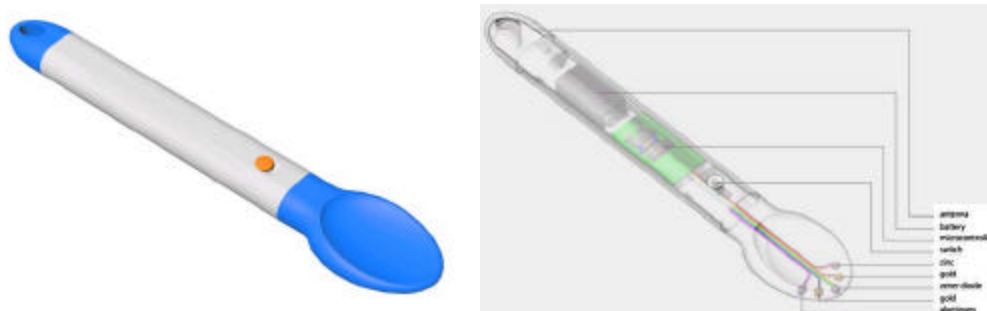
Figure 8: Final design of the spatula and a see-through rendition of the interior.
