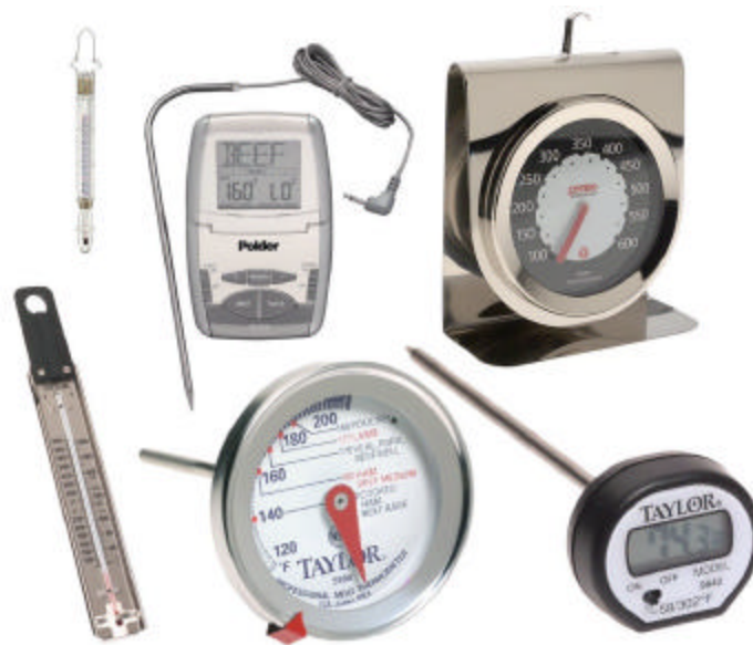
Figure 3: Kitchen thermometers. Clockwise from upper left: Matfer candy thermometer, Polder Preprogrammed cooking thermometer, Pyrex oven thermometer, Taylor digital instant-read pocket thermometer, Taylor professional meat thermometer, Taylor candy/jelly/deep-fry mercury thermometer.
