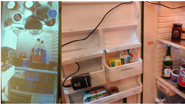
Figure 5. FridgeCam: projection on the refrigerator door (left), location of digital cameras (right).
