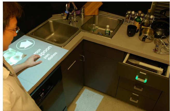
Figure 2. An example of endogenous cueing (left) and exogenous cueing (right) in the augmented reality kitchen.
