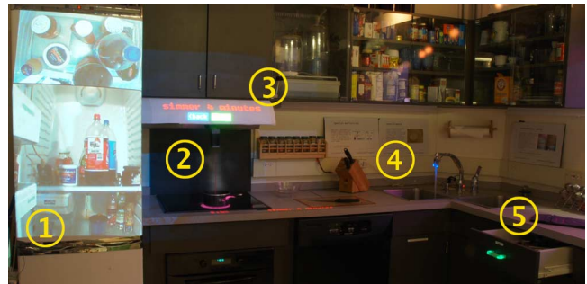
Figure 1. Augmented Reality Kitchen: information projection on the refrigerator (1), the range (2), the cabinet (3), the faucet(4) and drawers(5).
