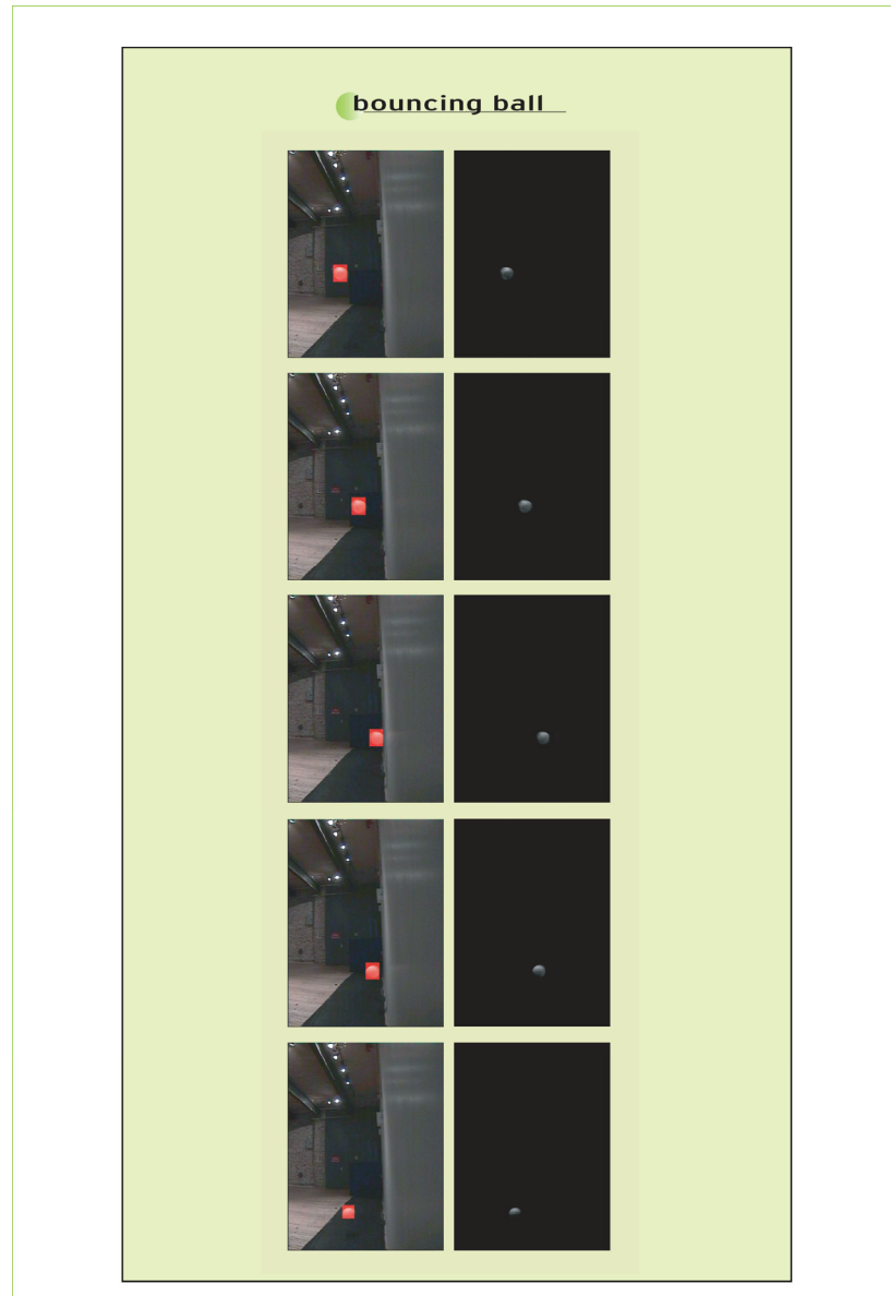
Figure 18 Ball bouncing off the wall, as seen from the side camera. On the right is the corresponding difference image.
