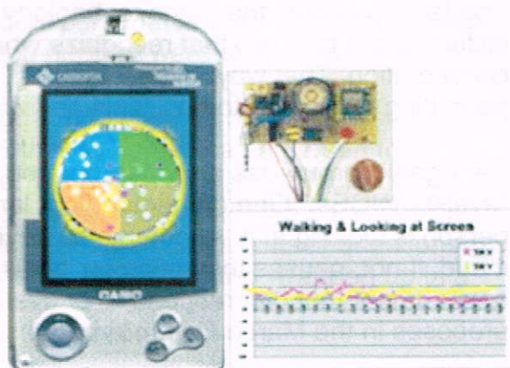
POCKET ROCKET. Sensor-packed personal digital assistant automatically recognizes certain user gestures. For example, holding the device to the mouth prompts it to record a voice memo. Horvitz
