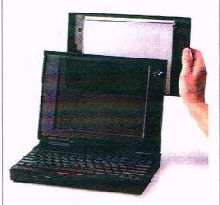
package, resulting in a laptop computer with the capabilities of a full-fledged multimedia workstation — all in a battery-powered presentation package weighing only 7.5 pounds. (See table for model comparison.)
