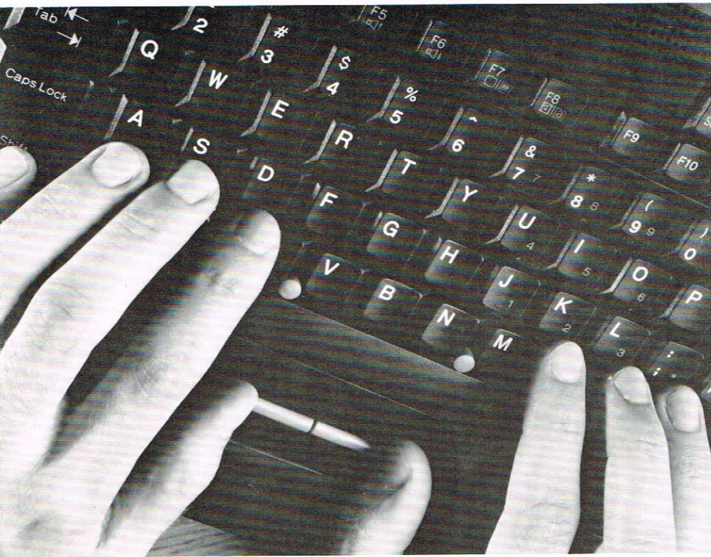
Two TrackPoints enable ThinkPad users to pick a function with one and perform it with the other.
