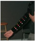
communication through arm motion. It consists of an analog force-sensing variableresistor measuring elbow position, a PIC computer, lights and an enunciator as effectors. Socially, arm motions are significant. When a person moves his arm wildly we stand back; when s/he waves we wave back. While
