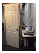
than Couch The Digital Threshold relies on two switches, one on the outside and one on the inside of the door. Coupling these switches to a voice recognition system and Microsoft Office the system counts the number of people in a room, notices whether a person has an appointment, identifies people, the occupant allows to respond, and updates and manages the office owner's
