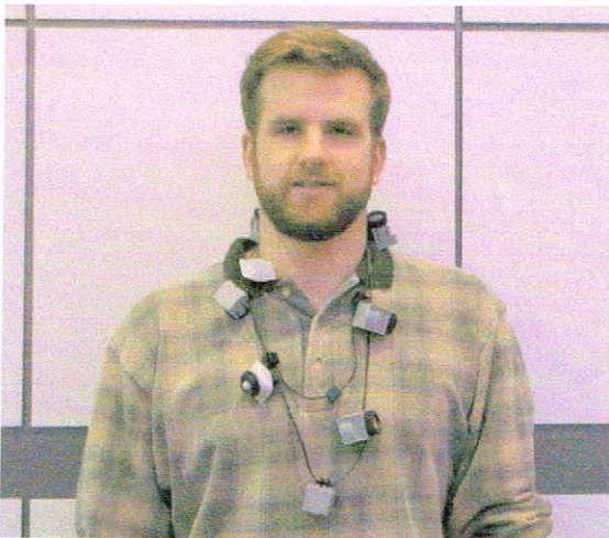
Figure 2 The Electronic Necklace, without a power source or computation, uses interaction with motors, lights, and sounds to create a baseline application for context-aware research.
