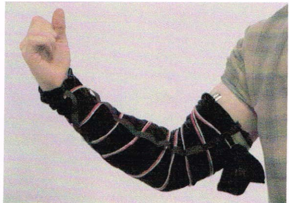
Figure 4 Flexor provides visual and audio feedback to motion for therapy and performance.
