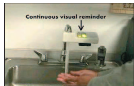
Figure 4: WaterBot offers continuous water usage feedback. It does not interfere with tasks performed at a typical sink.
