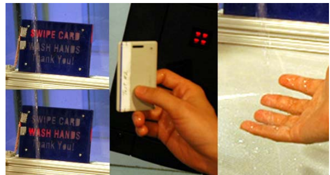
Figure 5. Clean Sink showing indicator (left) RFID reader (middle) and sink (right).
