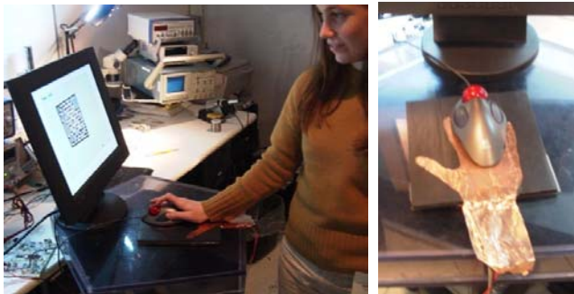
Figure 1. Thermo-mouse pad implementation. It warms a wide area in contact with the user's hand.
