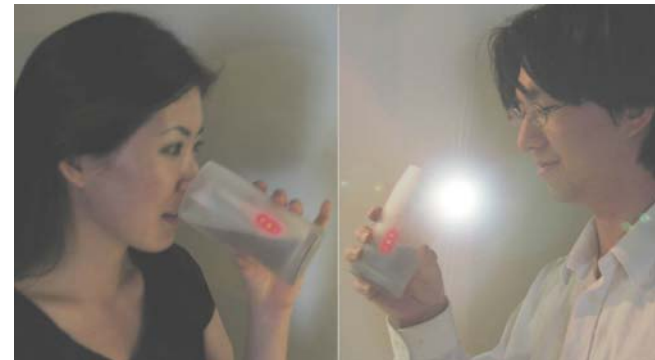
Figure 1: The Lover’s Cup in the right picture shows the liquid level of the other cup in the left picture while the other user is drinking. The top area of the cup is illuminated while the other user’s lips are touching the other cup.
