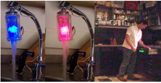
Figure 5. Colored illumination as a non-invasive display for temperature (left) and location (right).
