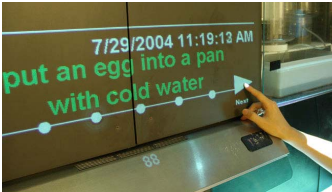
Figure 2. A step-by-step recipe with camera-based touch interface.
