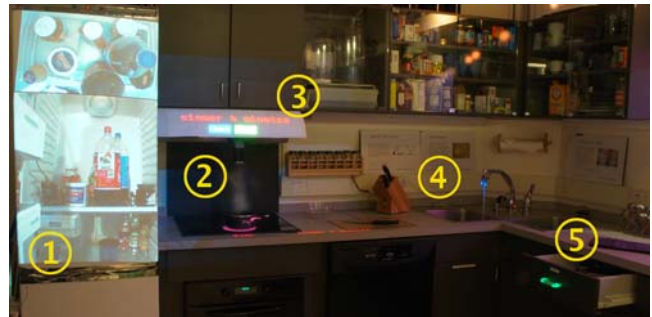
Figure 1. Information projection on the refrigerator (1), the range (2), the cabinet (3), the faucet(4) and drawers(5).
